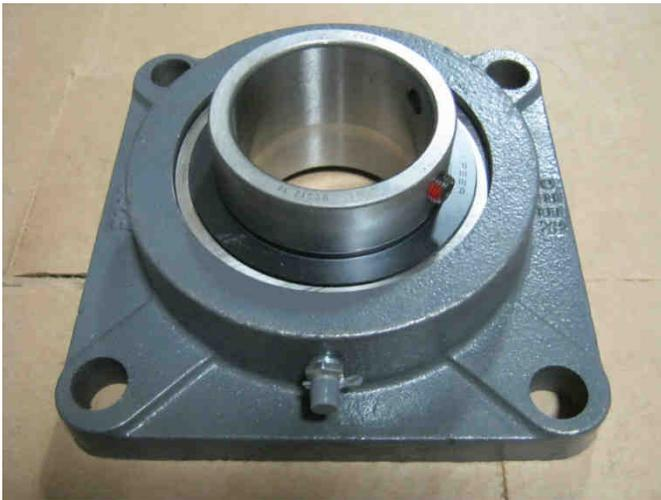
Image 3-11 – Bearing used on unload rotor
