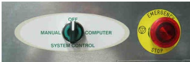
Image 11 – System Control switch and Emergency Stop switch
