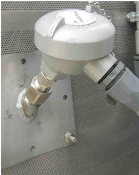
Image 14 – Single-point grain temperature sensor RTD
