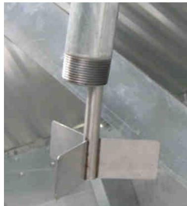
Images 4-2, 4-3 – Upper rotary fill switch, fill sensor
