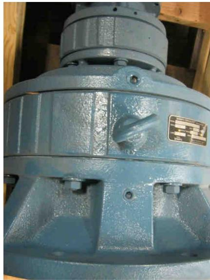
Image 3-9 – Shimpo gear reducer
