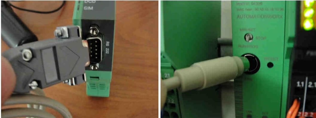
Images 4 and 5 – Connecting modem to PLC
