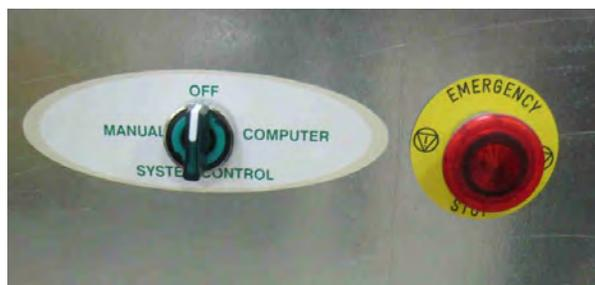
Image 3 – System Control and Emergency Stop switches
