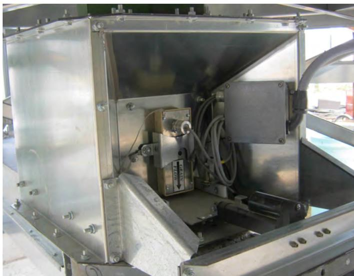
Image 4-10 – Discharge moisture sensor in static sample box
