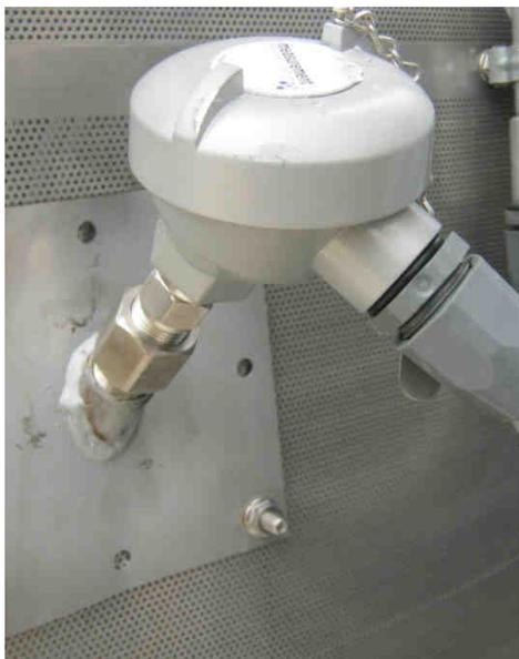
**Image 4-12 – Single-point grain column temperature sensor**
